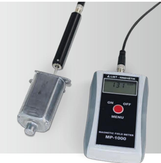
The **List-Magnetik MP-1000** magnetic field meter is a handy universal device with externally connectable tangential and axial field probes for the precise measurement of all types of magnetic fields: steady DC fields, alternating AC fields and pulsed fields.
